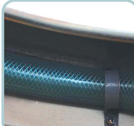
Water inlet and hose inside the drum helps flush feathers
