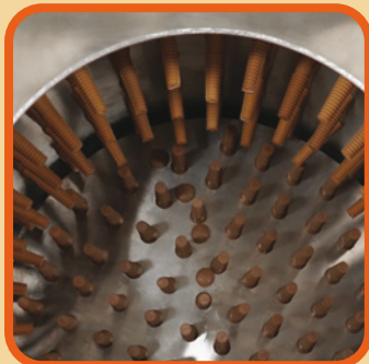
Drum has 196 plucker fingers for max efficiency
